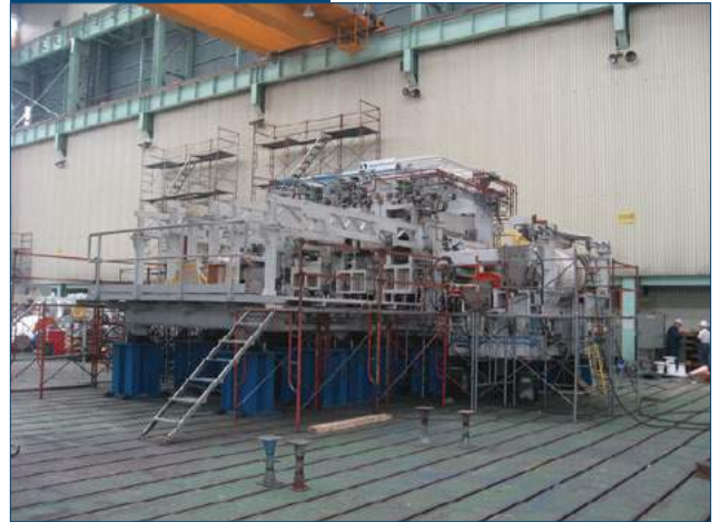
New tension leveler for advanced high-strength steel (AHSS).
