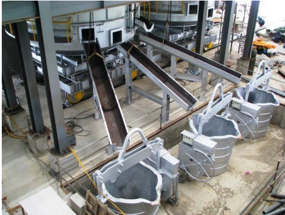
Fig.5 Furnace body and tapping troughs
